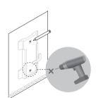
Place the mounting bracket in the right position. Mark two positions for the screw holes.
