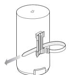
Lead the end of the pole mounting strap through the back of the Deco.
