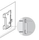
Insert the plastic wall anchors into the 6 mm diameter holes.
