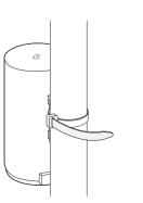
Position the Deco and wrap the pole mounting strap around the pole.
