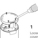
Loosen the screws to detach the waterproof cover of the Deco with a Phillips screwdriver.
